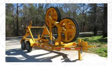
The TSE Model T50/52 BWRC Bullwheel tensioner/ reel carrier is designed to install single conductor or Fiber Optic Groundwire on transmission lines. Elastomer lined bullwheels with 1.5" grooves can handle conductors up to 1272 MCM and provide protection to delicate fiber cables. The bullwheels are tilted for groove alignment to eliminate any twisting being imposed on the cable. The lining segments are bolted on for easy replacement in case they are worn or damaged.
