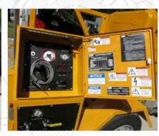
The TSE Model UP-85BD Underground cable puller provides infinite speed control and precise tension and distance monitoring. The 8" bullwheels are powered by a hydrostatic drive with a variable displacement axial piston pump and a two speed hydraulic motor. The cable payout is on demand with the bullwheel drive system feeding the pulling rope when any load in excess of 1 lb. is placed on the cable.
