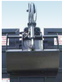
One-piece door with bucket rests available on certain models
