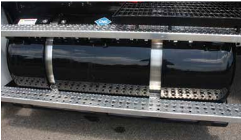
Pac-Mac can accommodate a variety of CNG tank options including below the rail saddle tanks or back of cab, above rail tanks
