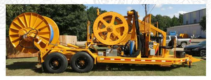
This compact traction unit performs equally well as a puller or a tensioner and is ideal for reconductoring applications. Having the self-loading, powered reel winder as an integral part of the machine allows reels of conductor or pulling rope to be loaded and unloaded without a crane on the location.
