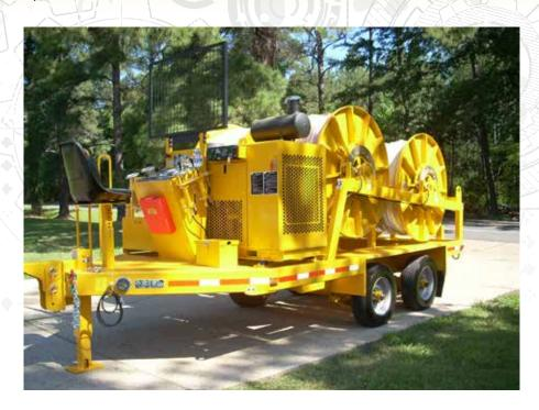
These four drum pullers with four separate pulling drums and ropes allow for the simultaneous or individual pulling in of three conductors and an earthwire.
