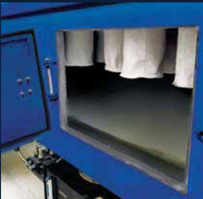
Larger baghouse access doors
