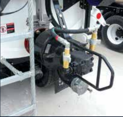
Rear door mounted sludge pump
