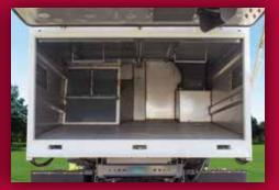
STAINLESS STEEL HOPPER SYSTEM This complete hopper body is constructed entirely of 304 grade stainless steel to provide maximum service life, even in the most corrosive applications. It is backed by a lifetime warranty\*.
